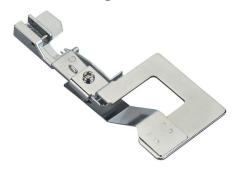
Another option for the overlocker is to use a gathering foot. The shape of this foot assists in holding the fabric to be gathered while also allowing for it to be sewn to a flat fabric. The fabric that is to be gathered should be underneath the foot against the feed dogs, while the flat fabric will slide between the foot and the bottom metal edge of the foot.
