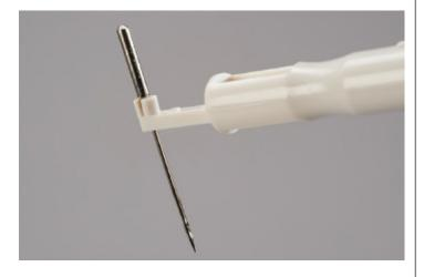
Use the needle inserter to hold the new needle in place while inserting and tightening the set screw.
