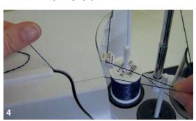
During the initial threading of the sewing computer and when the radial thread release is used it is advisable to pull an extra inch of thread from the spool before the threader button is pushed (Fig. 4).
