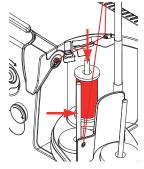
Any of the two spool pins (see arrow markings) can be used. However, it is best to use the rear pin due to its more favorable unwinding angle. Refrain from using the pin of the winder.
