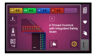
Follow the set up wizard to make sure that you make all the correct manual changes and test sew for a balanced overlock stitch.
