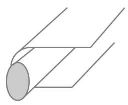
Using ¼" cording (cut two pieces) and two strips, wrap the strip around the cording leaving a tail of cording to place into the groove of the presser foot with raw edges of the fabric in front of the cutting knife.
